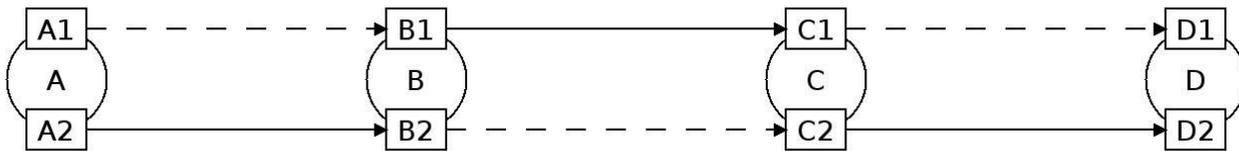
Interface alternating is performed by considering the interface where a packet has been received and choosing the best neighboring node of the available outgoing interfaces. On half-duplex interfaces like Wi-Fi forwarding decisions where sending and receiving interfaces are the same are considered worse and penalized to avoid possible selection.
